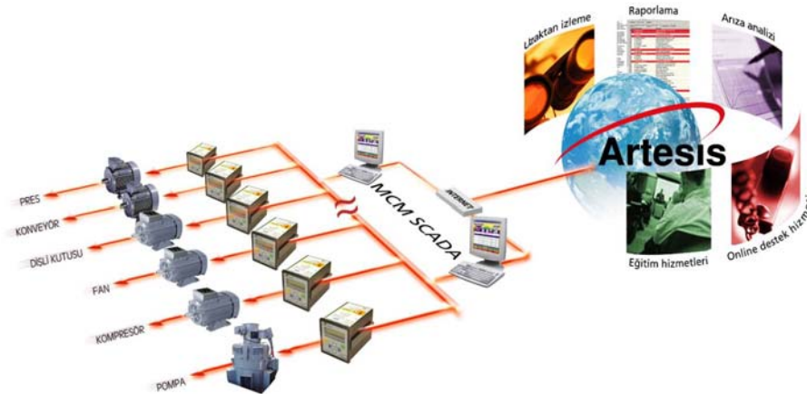
FIGURE 5 – MCM SCADA Network
